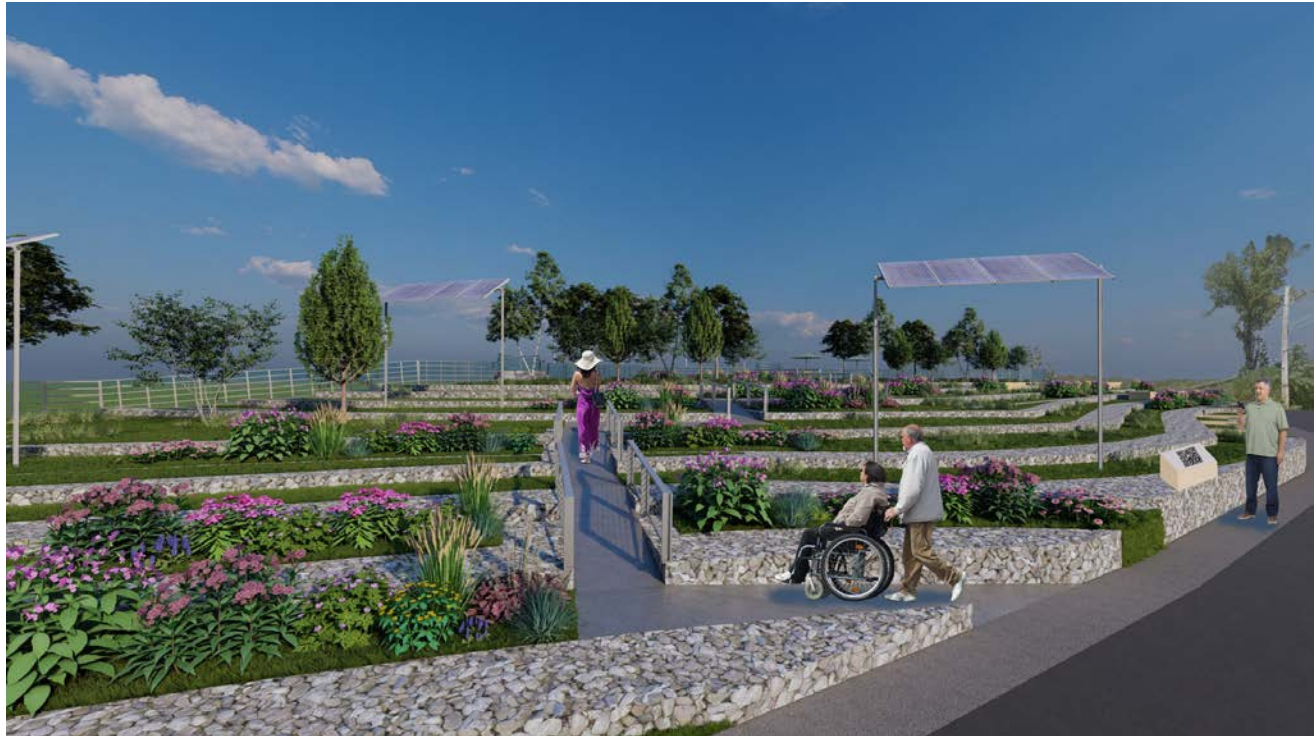
An ADA-compliant ramp series made from galvanized steel and trail surface aggregate works with the gabion terracing providing an accessible path to the top plaza.
